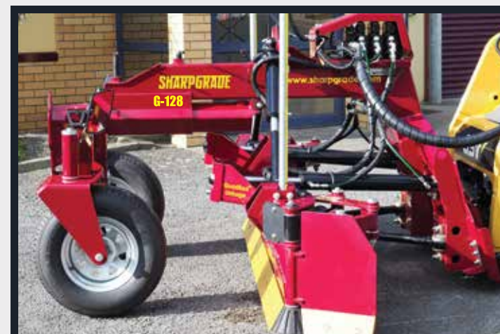
Retracting front chassis for reduced transport length
