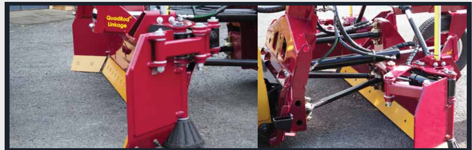
Cut, carry or windrow material forward or backward with double acting wings & rear blade
