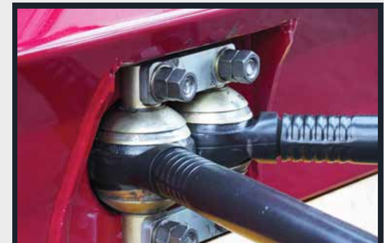
No grease All linkages are sealed for life
