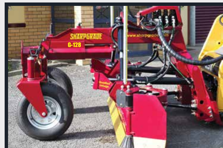
Retracting front chassis for reduced transport length
